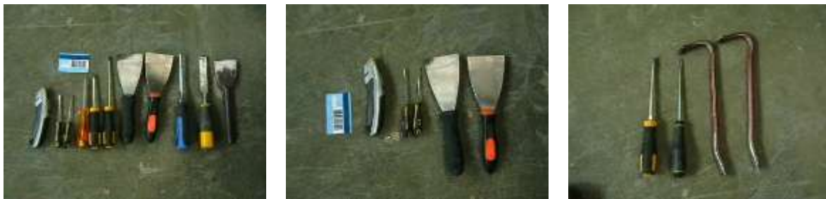
Figure 17 Tools specified in PAS 24 for glazing/infill panel removal (left), hardware manipulation (centre) and attempts to lever the door leaf open (right)
