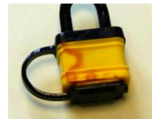
Water had penetrated via the shackle hole
