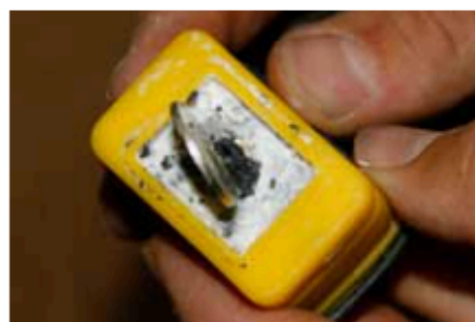
The lock had basically rotted from the inside
