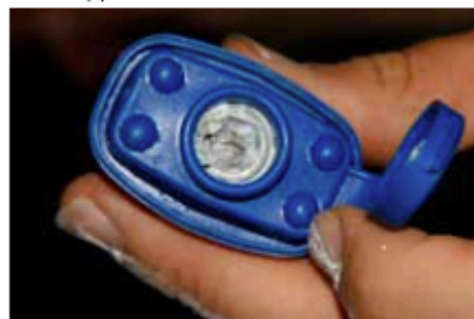
Internal corrosion after a month in the tank
