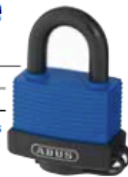
Result after a month in the salt spray tank
