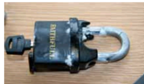
Result after a month in the salt spray tank
